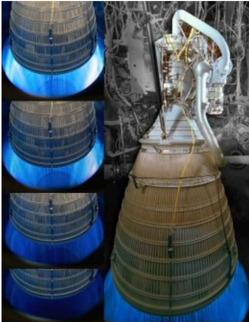
Multiple images on the left are pictures of the CECE engine at different throttle levels.
