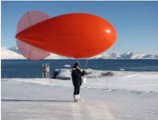
Jürgen Graeser with a tethered balloon for atmospheric measurements at the AWIPEV research Base. Photo: Heiko Gericke/Alfred Wegener Institute
