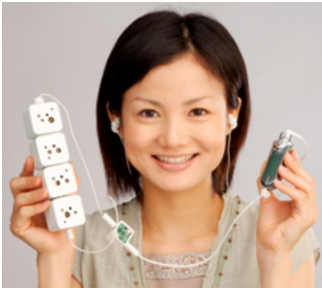
4 prototype bio battery units (left) connected to Walkman for playback. Credit: Sony
