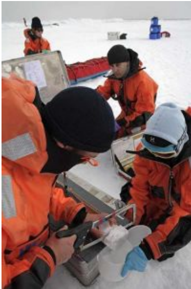
Scientists take ice cores for determination of sea ice thickness. Credit: Florian Brier/Alfred Wegener Institute
