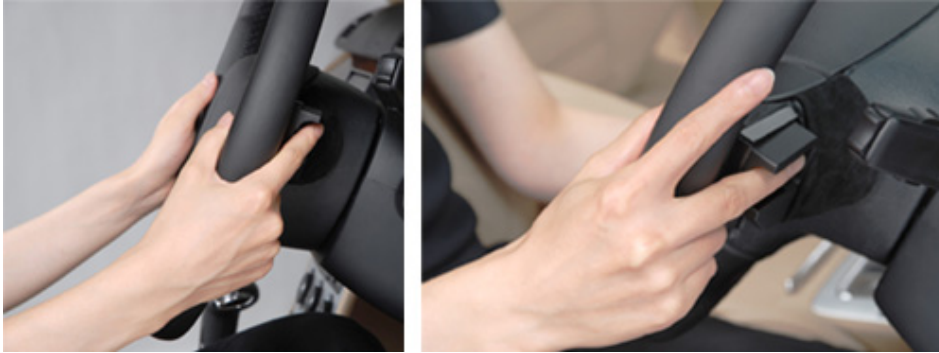
Finger vein authentication technology embedded on the steering wheel
