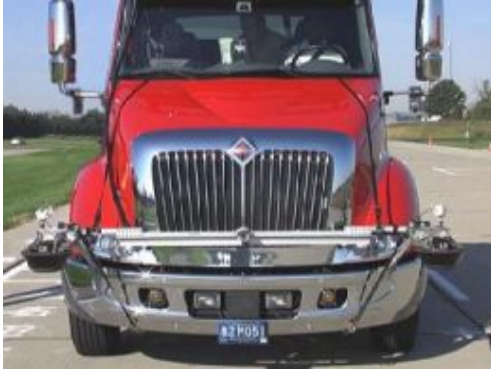
Truck cab instrumented for NIST tests of collision warning systems. Credit: NIST
