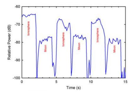
7.4075 Mhz signals from HAARP received by LWA on Oct. 28, 2007, 09:00 UTC. This figure shows the ionospheric reflections and the lunar echos of three of the more than 1400 HAARP pulses received by one of the LWA antennas in New Mexico. Credit: Naval Research Laboratory
