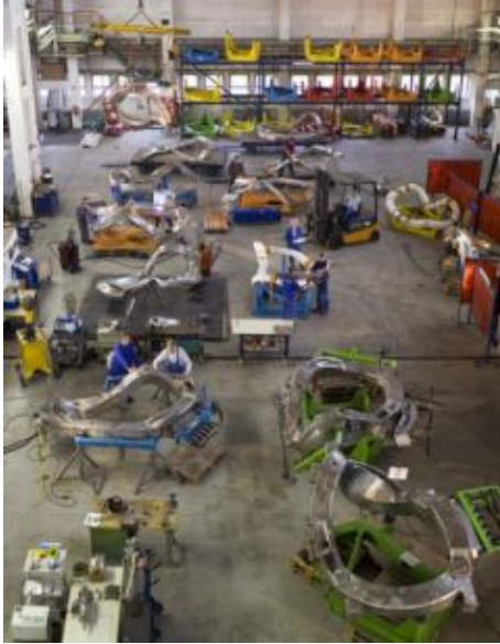
Final production of the magnet coils at Babcock Noell Magnettechnik GmbH in Zeitz. Credit: photo: IPP, André Künzelmann
