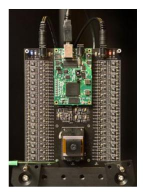
The testing platform for the multi-aperture image sensor chip.
