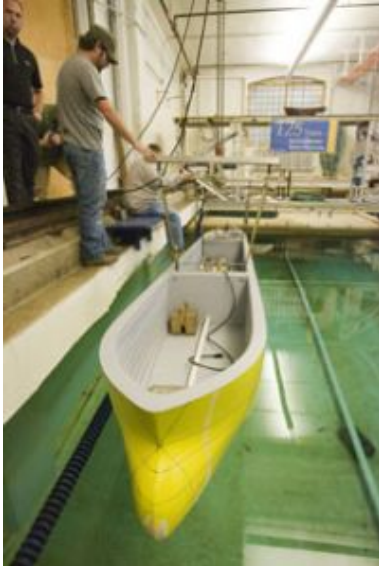
Workers lower a scale model of a Great Lakes bulk carrier into the towing tank at the U-M Marine Hydrodynamics Laboratory.
