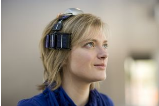
The wearable wireless EEG system with hybrid power supply.
