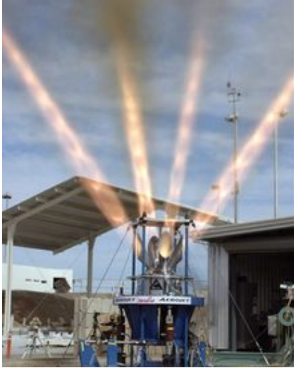
Orion Launch Abort System jettison motor test. Credit: AeroJet
