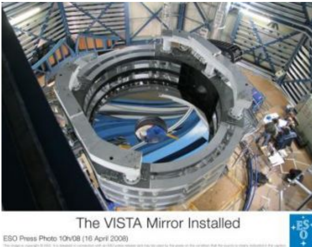
The 4.1-m coated VISTA mirror inside the telescope at Paranal. Credit: ESO
