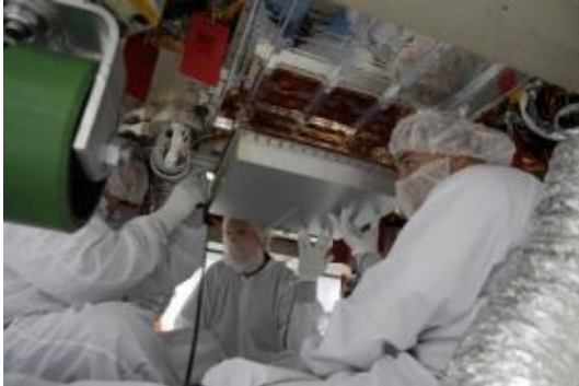
General Dynamics technicians, sitting under the GLAST spacecraft install a high-gain antenna on the spacecraft. Credit: NASA/ Kim Shiflett
