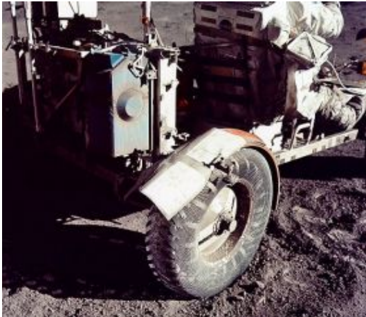
Apollo 17 moonbuggy fender repaired with duct tape.
