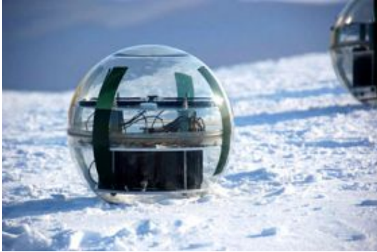
GPS buoys are used during the campaign to measure sea ice drift. They are deployed through planes or helicopter landing directly on sea ice floes. Credits: ESA
