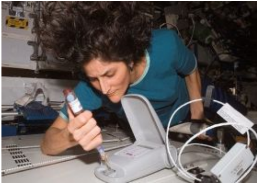
Astronaut Suni Williams (with flowing "microgravity locks" of hair) uses LOCAD-PTS onboard the International Space Station.
