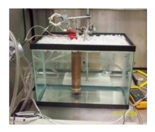
A new "calorimeter," shown immersed in this water bath, provides the first inexpensive means of identifying the hallmark of cold fusion reactions: the production of excess heat. Credit: Melvin Miles
