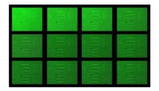
By adjusting an electrical voltage across a crystal of nonlinear material, the researchers recovered an image of lines and numbers that originally was hidden in noise (upper left). As they tuned the system (from left to right across each row from top to bottom), the image "stole" energy from the noise, first appearing and then degrading as they adjusted past the optimal voltage. (Images: Jason Fleischer/Dmitry Dylov)
