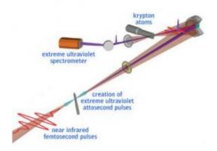
Femtosecond-scale pulses were fired to ionize krypton atoms (wide beam). Separately created attosecond-scale pulses (narrow beam) were absorbed by the
