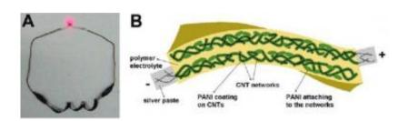
(A) Using three of the new highly flexible supercapacitors arranged in series, the researchers demonstrated lighting a red LED. (B) An illustration of the flexible, all-solid-state paper-like polymer supercapacitors. Image credit: Chuizhou Meng, et al. © 2010 American Chemical Society.
