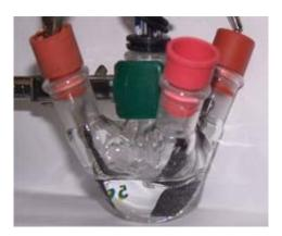
An electrode made of a copper- and iron-based nanomaterial is immersed in a potassium nitrate electrolyte. Image credit: Colin Wessells, et al.
