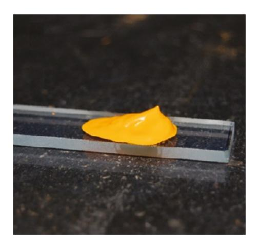
Application of solar paint to an optically transparent electrode. Image credit: Mathew P. Genovese, et al. ©2011 American Chemical Society
