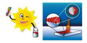
Titanium dioxide nanoparticles are coated with CdS or CdSe. The composite nanoparticles, when mixed with a solvent, form a paste that can be applied as one-step paint. Image credit: Mathew P. Genovese, et al. ©2011 American Chemical Society
