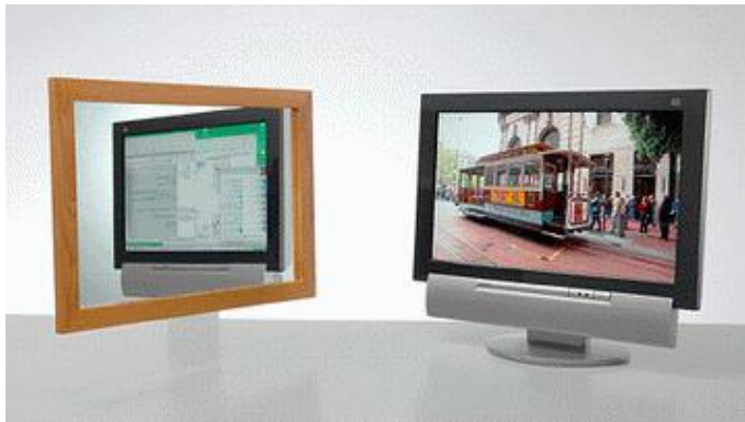
Two-way viewing-angle LCD (26-inch LCD IT-TV prototype) Reflecting the LCD in a mirror shows that one user sees TV images from the right while another can see an Internet home page from the left.
