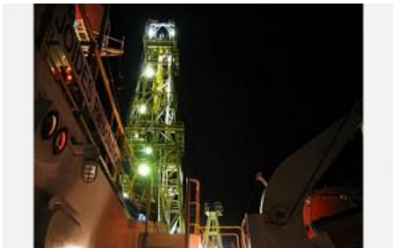
The derrick of the JOIDES Resolution, the scientific drilling ship used to recover the intact section of ocean crust. Credit: IODP
