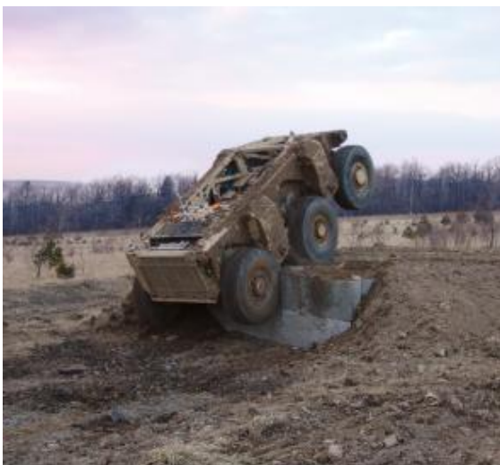
Crusher can climb > 4 foot steps
