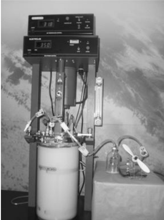
Coupling of Bio-H 2 made by fermentation of confectionery waste to the operation of a PEM fuel cell used to drive an electrical device.
