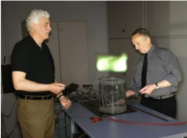
A ball-lightning-like plasma cloud is produced in an underwater discharge. (Photo: D. Lange, IPP)
