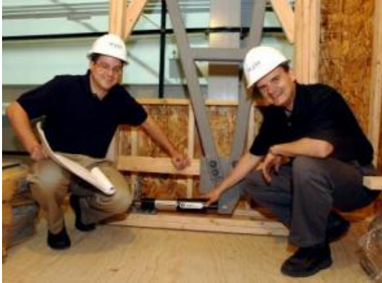
Michael Symans of Rensselaer (left) and Andre Filiatrault of the University at Buffalo with the seismic damper installed inside a bedroom wall of the NEESWood townhouse. Credit: University at Buffalo/Parisi
