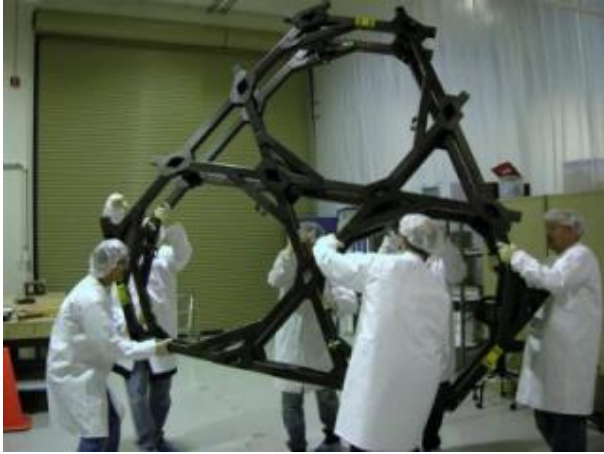
Scientists and Engineers at Northrop Grumman working with the Backplane or "spine" of the JWST. Credit: Northrop Grumman
