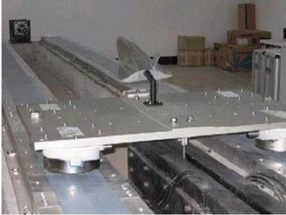
Model of the maglev launch assist: a 40 kg vehicle was accelerated to 5 m/s on the seven meter track. Credit: Wenjiang Yang, et al.
