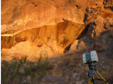
The LIDAR instrument (foreground) scans an exposed fault, measuring its topography in great detail. Photo by A. Sagy
